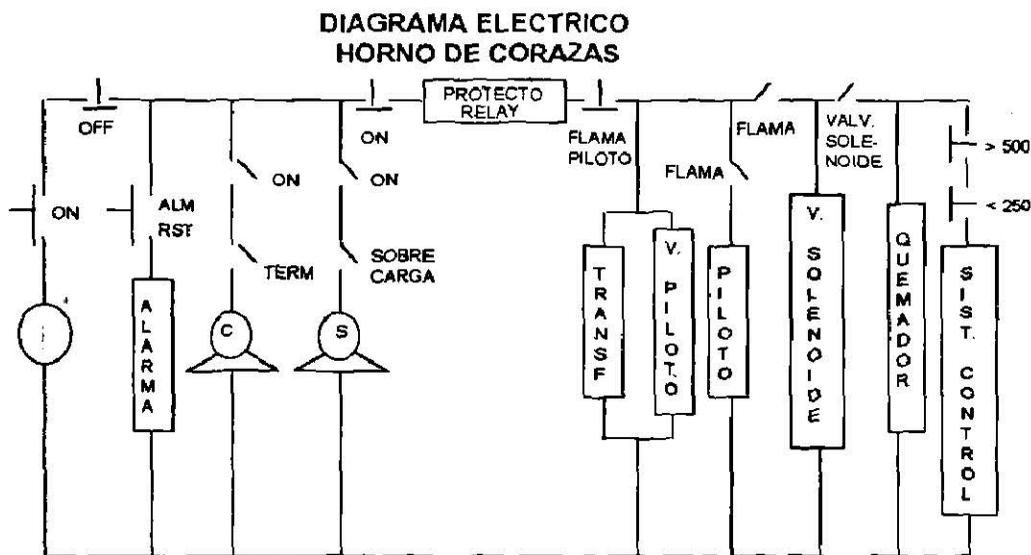
FIG. 2: DIAGRAMA ELECTRICO DEL PROCESO
